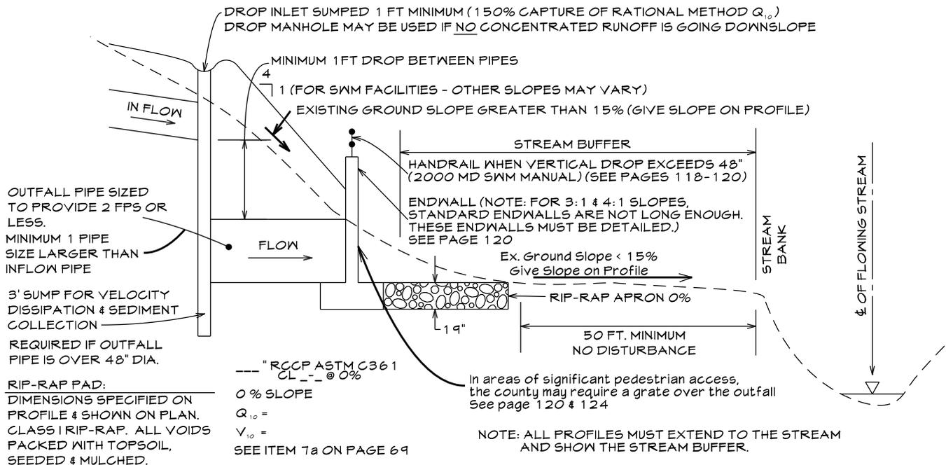
IF: THE DROP STRUCTURE AND OUTFALL PIPE ARE CONSTRUCTED AS SHOWN ABOVE, THEN: THE OUTFALL MEETS THE 2 FT/SECOND CRITERIA FOR DISCHARGES UP TO THOSE FOUND IN TABLE 2
