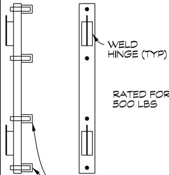
**CONTINUOUS PLATE HINGE DETAIL**
