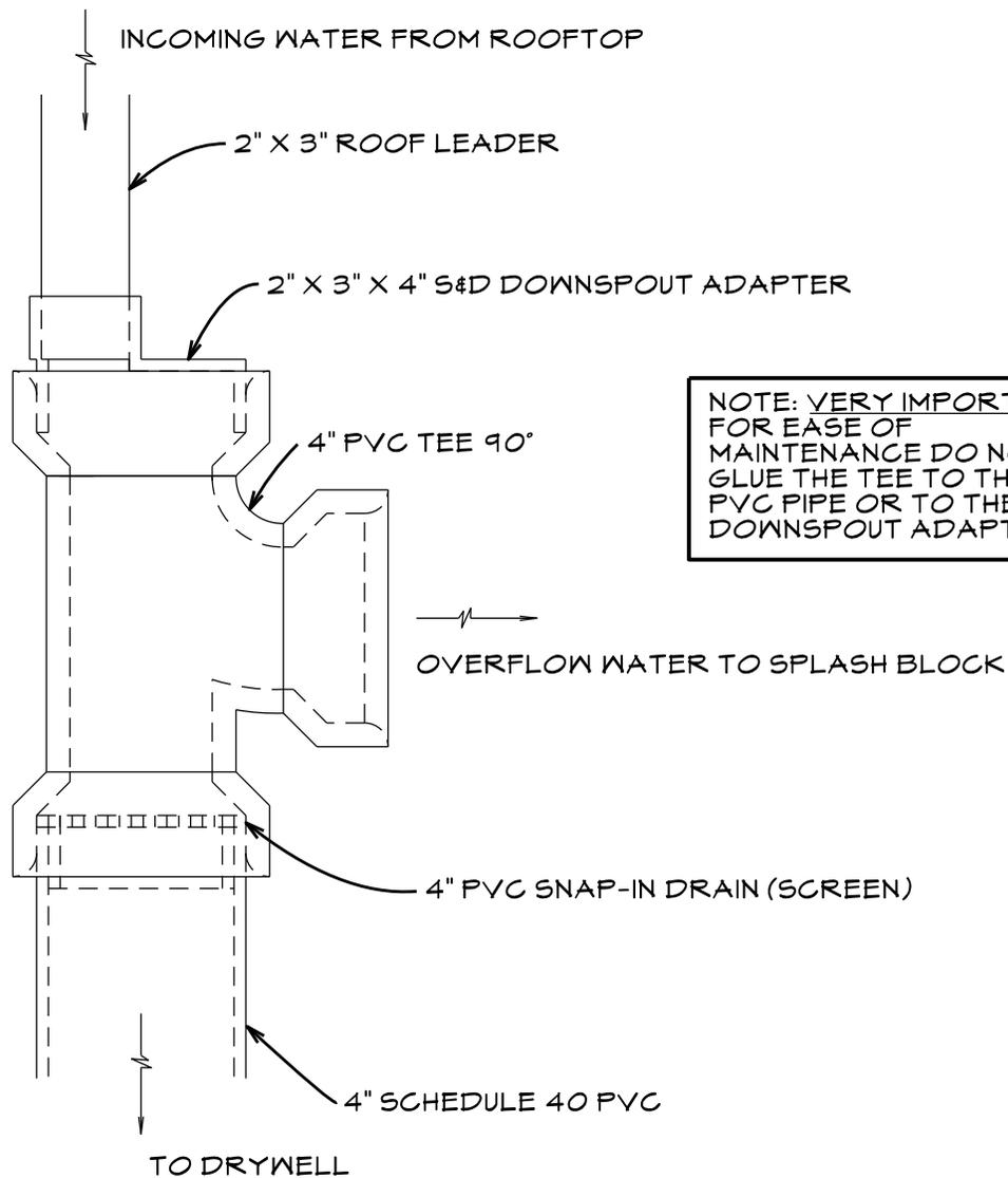
NOTE: VERY IMPORTANT FOR EASE OF MAINTENANCE DO NOT GLUE THE TEE TO THE PVC PIPE OR TO THE DOWNSPOUT ADAPTER.
