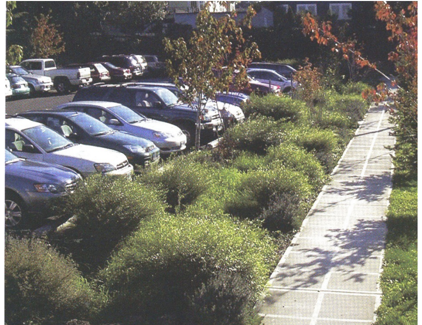
(Above) Raingardens allow for the infiltration of stormwater runoff and can be attractive landscaping elements in and of themselves. (P.E.L.A.)
