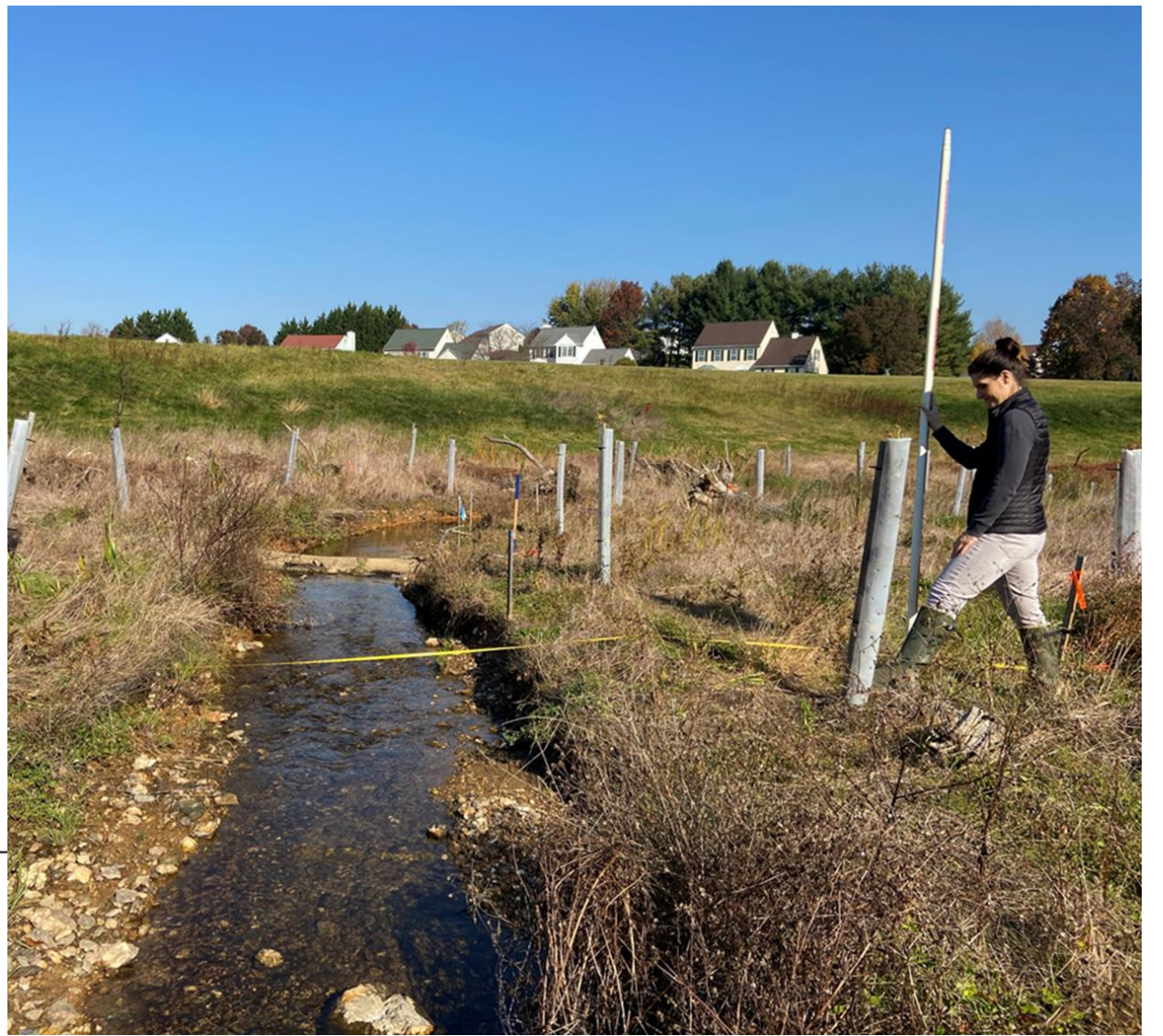
Measuring Erosion-Elevation Surveys
