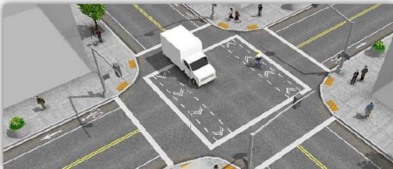
Figure 7-19: Intersection Crossing Markings, NACTO p. 137
